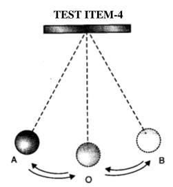
A simple pendulum consists of a small metal ball called bob which is suspended by a long thread from rigid support such that bob is free to swing back and forth. The to and fro motion of a simple pendulumis an example of periodic or oscillatory motion. Galileo was the first person to study the motion pendulum.
