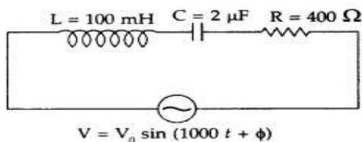
(ii) Without making any other change, find the value of the additional capacitor  $C_v$  to be connected in parallel with the capacitor  $C$ , in order to make the power factor of the circuit unity.
