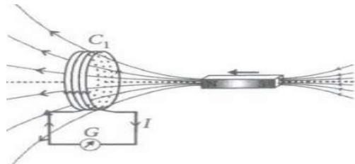
(i) The north pole of a long bar magnet was pushed slowly into a short solenoid connected to a galvanometer. The magnet was held stationary for a few seconds with the north pole in the middle of the solenoid and then withdrawn rapidly. The maximum deflection of the galvanometer was observed when the magnet was -
